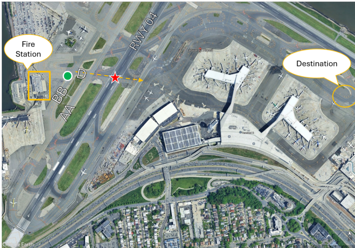
Figure 1. Google Earth image of the accident area, with the green circle indicating where the ground vehicles initially gathered, the yellow dash line their intended path on taxiway D, and the red star indicates where the collision occurred.
