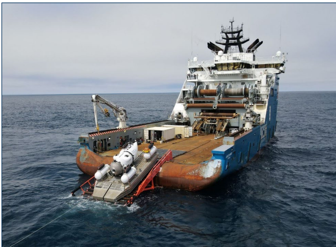
Figure 8. The Titan and LARS being launched via stern ramp from the Arctic Horizon in 2022. (Source: Garry Comber)
