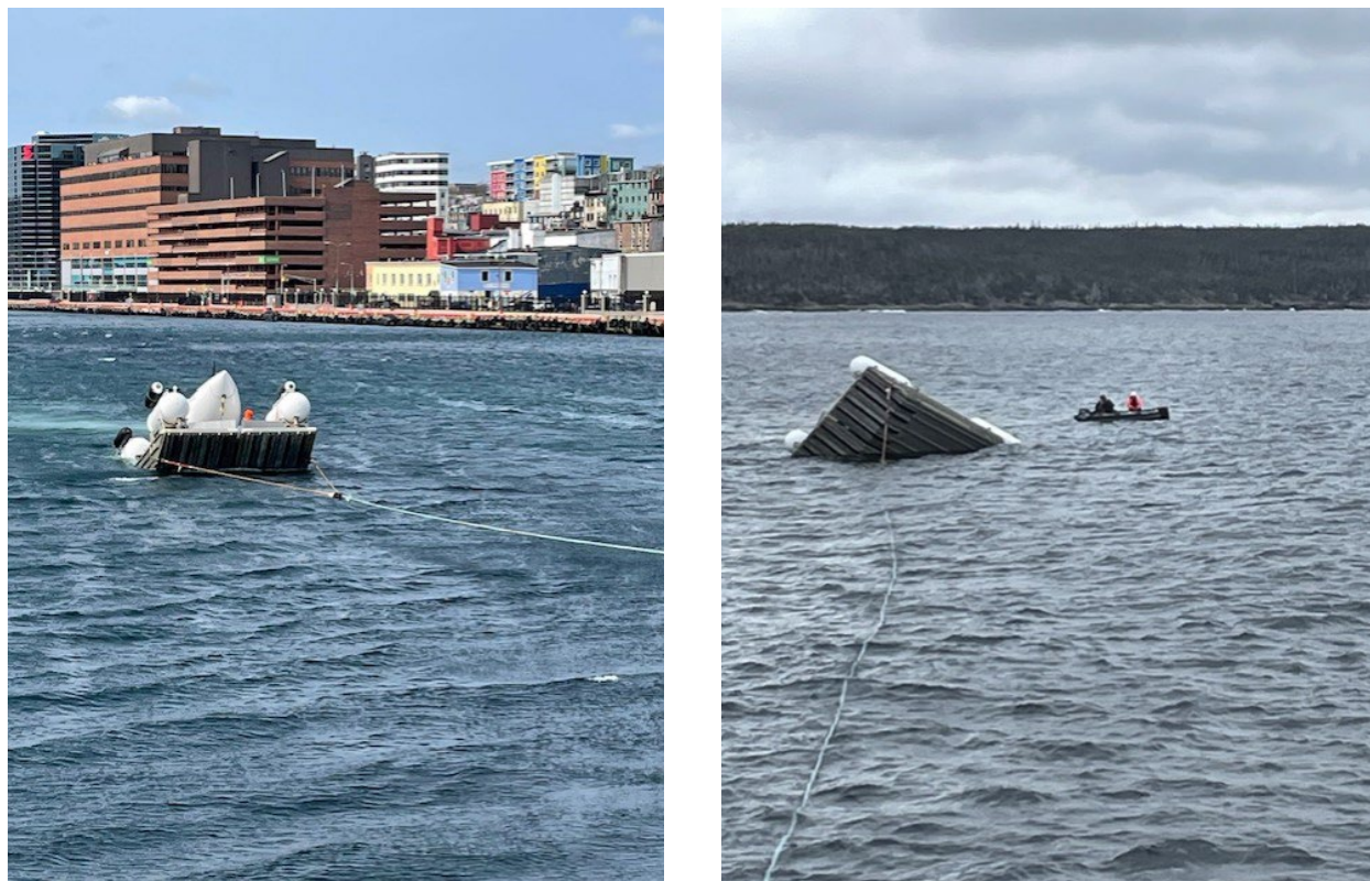
Figure 10. Left to right: Operational mishaps during the 2023 expedition showing the aft starboard corner of the LARS tipped downward on May 20 while leaving St. John’s, and the aft end of the LARS tipped downward on May 27 in Witless Bay, Newfoundland and Labrador. (Source: Steven Taragel)
