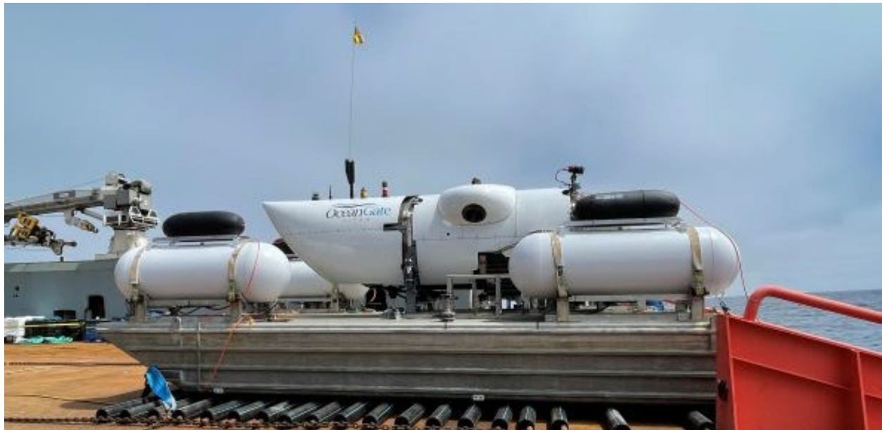
Figure 4. From top: Top-down view of Titan on LARS (scale approximate), and Titan secured on LARS in 2022. (Source [bottom]: Garry Comber)
