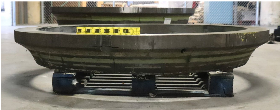
Figure 15. Side view of a trimmed end piece of the Titan cylinder.
